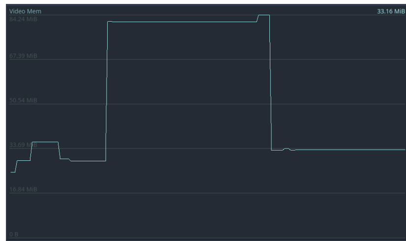
Figure 5.2: Graph detailing the VRAM usage of the game over the course of 1 match
