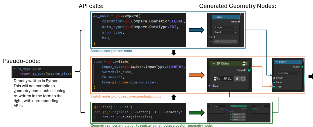
Figure 3.6: Usual logics cannot be written in Python directly, such as if-statements. They need to be expressed in the same way as if it is implemented in geometry nodes directly with built-in nodes. Green part also shows how to register a Python method as a custom geometry node.
