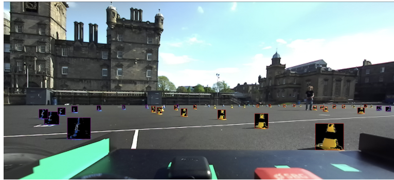
Figure 3.2: EUFS-AI camera image with cone extraction algorithm.
