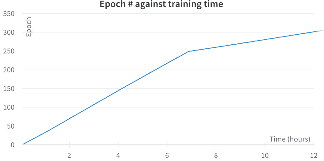
Figure B.1: The fixed implementation of CodeNeRF executes 300 epochs in 12 hours when trained on 14 models. The difference in gradient is due CodeNeRF’s cropping routine. The first 250 epochs are trained on 64 \times 64 centercrops, the rest on the full 128 \times 128 images. For each model, 50 out of 250 viewpoints were used, in accordance with CodeNeRF.
