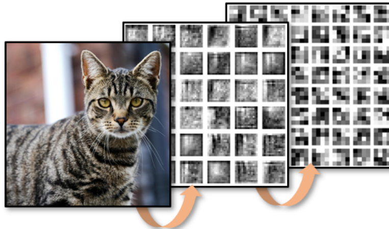
Figure 2.3: Hierarchical feature decomposition through feature learning in deep CNN. Left to right: input image, first layer and last hidden layer's feature maps of the image.
