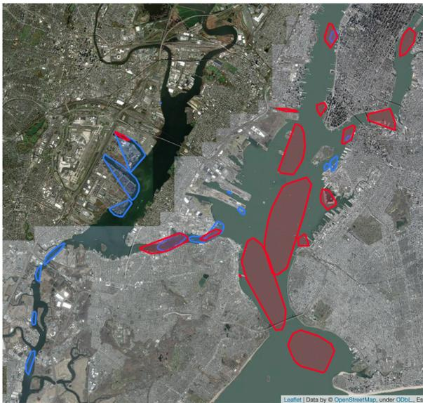
Figure 5.2: Port of New York region identification (berths in **blue**, anchorages in **red** )
