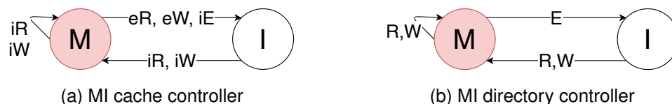
Figure 2.1: MI protocol. Legend: R = Read; W = Write; E = Eviction; i = internal (originating in the machine itself); e = external (originating in some other machine).
