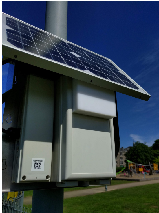
Figure 3.1: The stationary AIRSpeck sensor uses a solar panel for power and can be affixed to common street furniture such as a pole or lamp post as shown.
