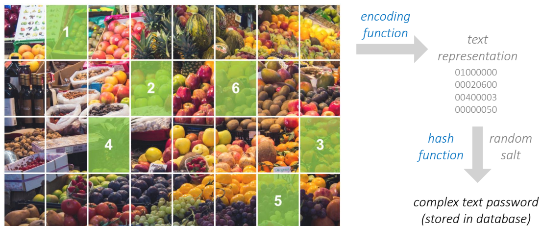
Figure 5.5: Graphical password encoding and encryption
