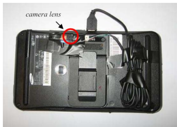
Figure 3: Back of Samsung minicomputer with attached camera for video processing
