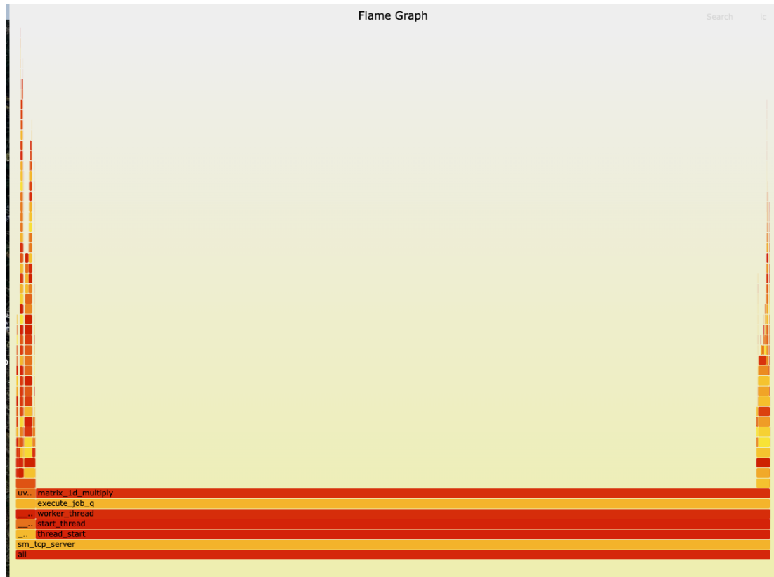
Figure F.1: Flame graph of the call graph at one of the Raspberry Pi nodes. Zoom out to show the prevalence of the multiplication task
