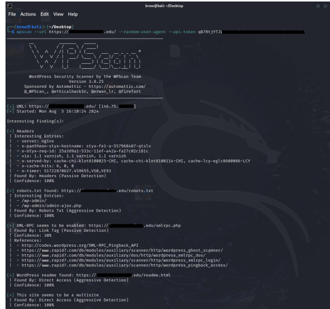
Figure 4.1: WPScan [86] detecting vulnerabilities on a website
