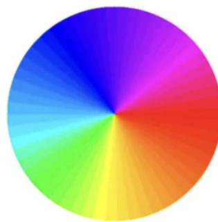
Figure 2.2: Color Wheel used for representing optical flow [10]
