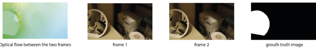
Figure 2.4: The leftmost image is the optical flow image generated by the RAFT model; the middle two images are random consecutive frames, and the rightmost image is the ground truth mask showing the segmentation mask for the mirror. The optical flow image (leftmost image) shows there is a clear boundary between the motion of objects inside the mirror and its immediate surroundings
