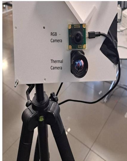
Figure 3.1: Platform with RGB and Thermal sensor
