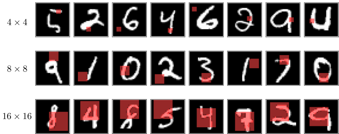
Figure B.1: Uniform random sampling patch examples - patch samples, \pi_t , coloured in red, sampled from MNIST images using random sampling introduced in Section 3.2.1 for patches of size 4 \times 4 , 8 \times 8 and 16 \times 16 .
