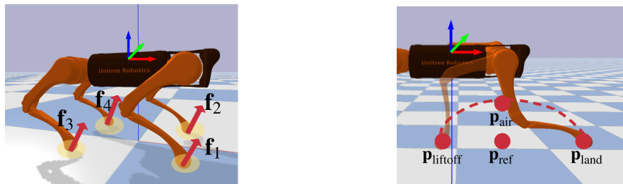
(a) Stance controller, optimizing the ground reaction forces [65] (b) Swing controller, producing parabolic foot position trajectories [65]
